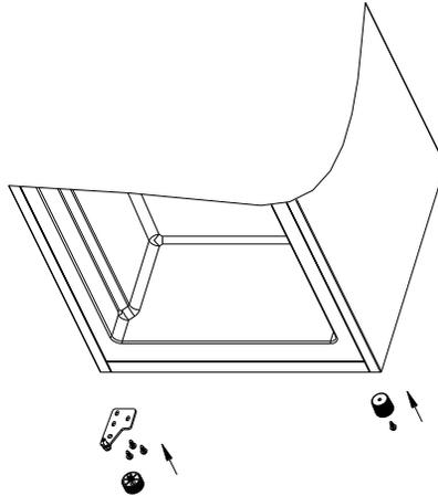
7. Assemble the door and top cover. Fix the top cover by screws and fix the screw cover.
