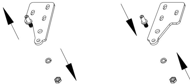
6. Using the screws to assemble the lower hinge at the right.,assemble the adjustable foot. Using the screws to assemble the front foot at the left.
