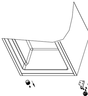
5. Remove the nut of the lower hinge, remove the spring and pin. Then turn over the lower hinge. Using the nut and spring to fix the pin.
