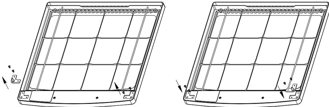
3. Remove the door. Take out the sleeve from the top of left door, and plug from top of right door. Then put the sleeve into the top of right door and plug into the top of the left door.
