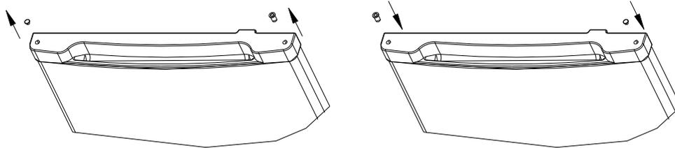
4. Remove the adjustable foot from the bottom of the unit. Remove the screws, and the hinge from left and remove the front foot from left.
