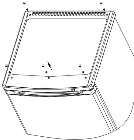
2、 Turn over the top cover, remove the screws. Fetch the hinge from the left side of the top cover, and use the screws to assemble the hinge into the right side of the top cover.
